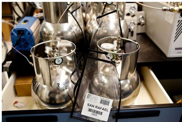
The canisters that were deployed during and after the Chevron fire to collect air samples to be brought back to the lab for testing at the Bay Area Air Quality Management District lab in San Francisco, Calif., Thursday, August 16, 2012. Photo: Jason Henry, Special To The Chronicle / SF
