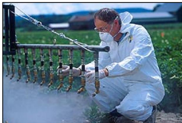
**Proper selection of spray nozzles can reduce drift by producing larger droplets.**
