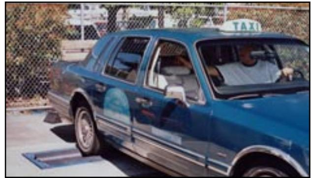
**County Inspectors can test taximeters in several different ways. Using a dynamometer allows very accurate test results.**
